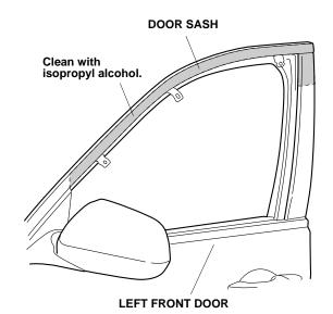
8. Position the left front door visor on the door sash. Push the front retaining bracket behind the door mirror base as shown.
