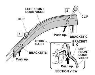
10. Adjust the position of bracket C and install the rear clip. There should be no clearance between the bracket and the door sash.
