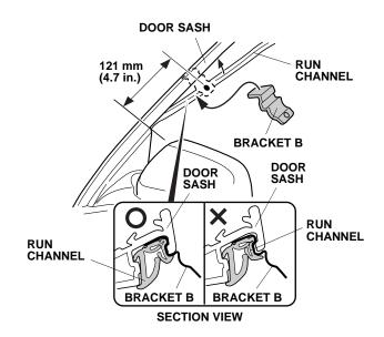
4. Position bracket D on the door sash as shown, then reinstall the run channel in this area.
