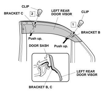
22. Adjust the position of bracket C and install the front clip. There should be no clearance between the bracket and the door sash.
