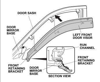
9. Adjust the position of bracket B and install the front clip.
