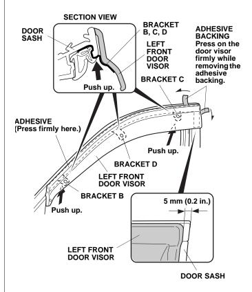
12. Press the left front door visor firmly against the door. Starting from the rear edge of the door visor and working forward, remove the two adhesive backings and attach the adhesive strips on the left front door visor to the door sash. With a soft towel around your finger, push up the brackets so there is no clearance between the bracket and the door sash. 13. Using one clip and one washer, secure the left front door visor to bracket D as shown.
